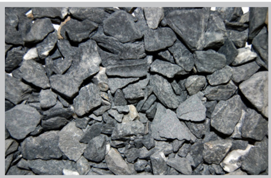
Single Chip Seal Aggregate (irregular size & elongated aggregate)
