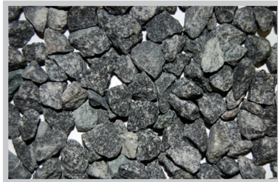
Single Size Cubical Aggregate utilized in High Performance Chip Seal
